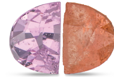
Lattice diffusion changed this pink sapphire to orange
